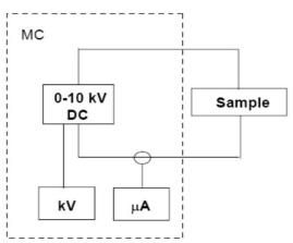
Standard measuring procedure: voltage rise from 1 kV .. [1 kV] .. 8 kV Current measurement for each voltage step after 1 min
